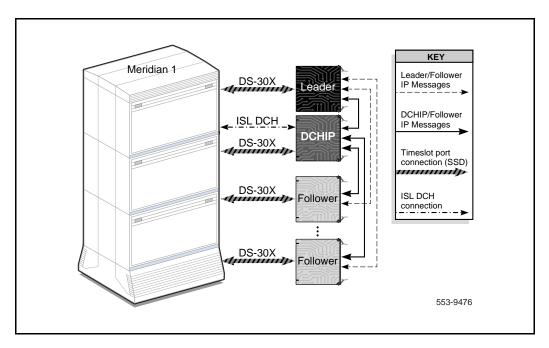
In Figure 9, the DS-30X connection is part of the Meridian 1 IPE shelf's backplane. The ISL DCH connection is a cable that runs from the "octopus" breakout cable, on the back of the IPE cabinet, to one of the MSDL's RS-422 ports. The Leader/Follower card messages normally travel over the T-LAN. The DCHIP messages travel over the E-LAN: a 10BaseT LAN connected to each ITG ISL Trunk card and the MAT PC. A separate 10/100BaseT LAN transmits the voice/fax data to the remote VoIP systems.
